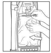
Make sure dirt inlet goes completely into dustbag and bag is pushed completely back into place. Tuck excess bag into cleaner.
